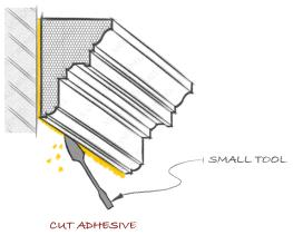
Then using the flat end of the small tool, scrape 'forwards', cleaning off any remaining adhesive (refer to the following diagram for scraping 'forwards'). This is important because scraping in the wrong direction presses the adhesive into the wall. The correct method will leave the remaining adhesive 'lifted', allowing for easier cleaning.
