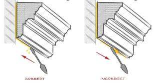
Using water and the 50mm brush (or sponge) clean away all remaining adhesive. Do not leave a groove between the moulding and the wall, as this will show up when painted. A flush corner with no surface adhesive is the ideal result, for the best finish.
